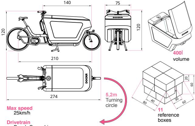
Bosch Cargo Line Enviolo Heavy Duty with AUTOMATIQ® shifting Gates belt drive
